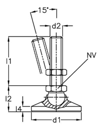
A/F = 15 d1 = 50 d2 = 10 l1 = 63 l2 = l4 = -Static load (N) = 11 Weight in (g) = 215
